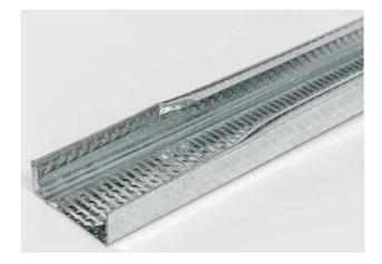
The branders are fixed with suspension brackets perpendicularly to the roof supports at no more than 400mm centres apart. The suspension brackets may not be more than 1.2m apart to support the steel branders adequately. It is recommended that a 20X20mm galvanised angle is to be installed at the perimeter to support the brander ends. Plasterboard is fixed at a right angle to the branders i.e. parallel to the trusses with 25mm drywall screws at centres not exceeding 150mm.
