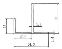
Used to create a neat finish on the corner of a bulkhead between the vertical and horizontal plain.
